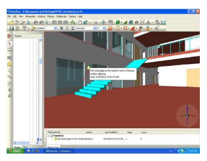
Figure 1: Add comments to building and facilities models during 3D Walkthrough
