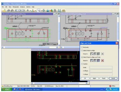
Figure 3: Compare two versions of a drawing and optimize revision processes with AutoVue
